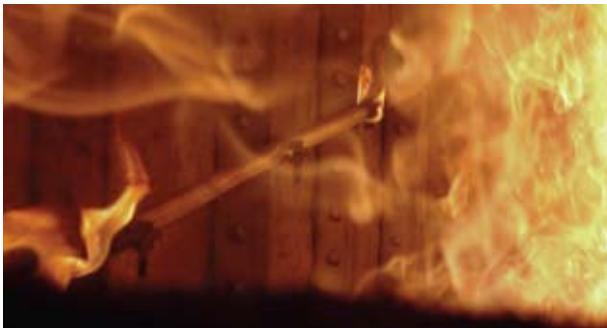
Lifeline undergoing UL 2196 testing
