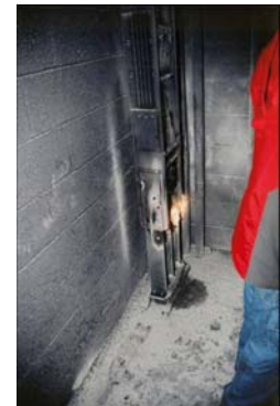
Figures 1(a) and 1(b): Melted copper buss and other debris on the floor
