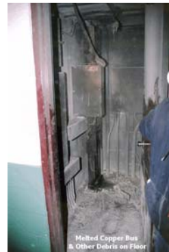
Figures 1(a) and 1(b): Melted copper buss and other debris on the floor
